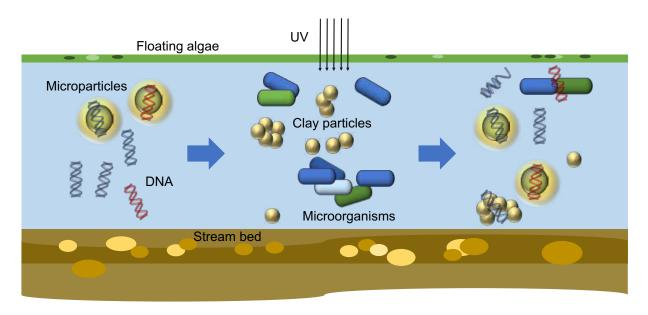
Fig. 4. / Transport of the free and microencapsulated DNA tracers in a surface water stream.
