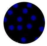
*Cryptosporidium* surrogate microparticles diameter 4.92 (± 0.04) μm
