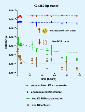
**Fig. 6.** / Degradation of free and microencapsulated DNA tracer in stream-water and dairy-shed effluent.
